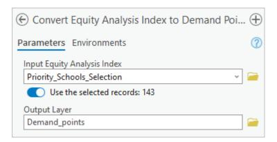
The tool provides a note that 143 records will be processed. This aligns with the number of records you were expecting based on the query you used in the **Select by attribute** tool.
