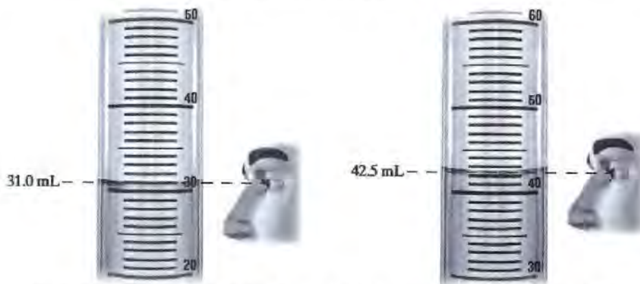
Figure 2.1 Graduated Cylinder Example readings using proper eye position and recording the bottom of the meniscus to half a subdivision ( \pm 0.5 mL).
