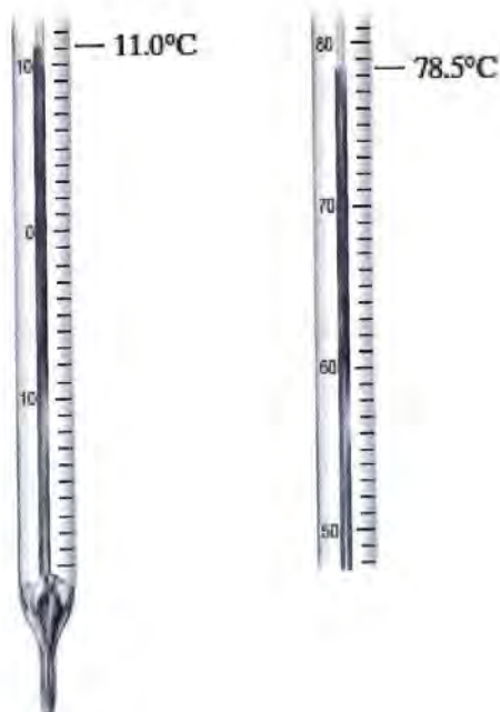
Figure 2.2 Celsius Thermometer Example readings using a Celsius thermometer and recording the top of the liquid to half a subdivision ( \pm 0.5 °C).
